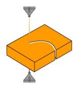
For wire cutting the required cutting form is stored or preprogrammed. Then the machine automatically cuts the form set in advance. Even complicated sloping or conical cuts are possible because of the independently working upper and lower wire guide. The proceeding is mainly used for the manufacturing of cutting and punching tools for the sheet metal industry.
