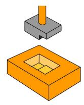
For sink erosion the required form is reproduced with a tridimensional electrode. This creates a negative of the final product. This procedure is used for manufacturing of forms for plastic parts like telephone casings, screw-type caps for bottles, forms for yogurt cups, spectacle frames and many other things.
